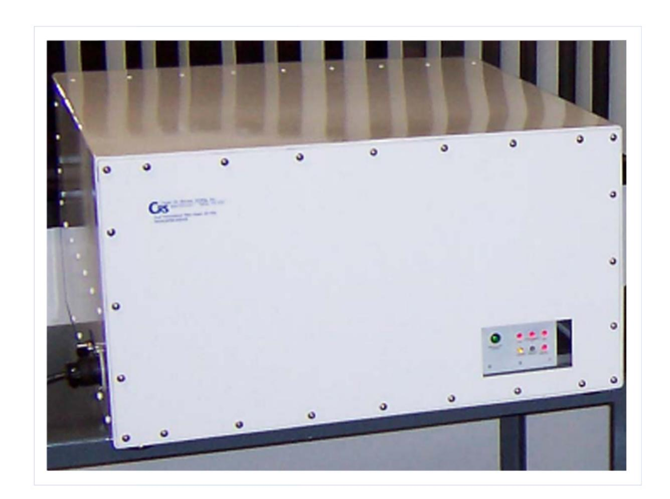
The radar parameters (Inter Pulse Periods (IPPs), Tx pulses, waveforms, sampling region, sampling rate, etc.) can be changed by the user using a menu driven interface. The radar can be operated with various types of waveforms (Pulse, FM, Phase Coded, etc.). Each IPP can be selectively defined. A sequence of IPPs are grouped as frames. A frame may consist of any number of IPPs of various types. The data for each IPP are separated in different buffers.
