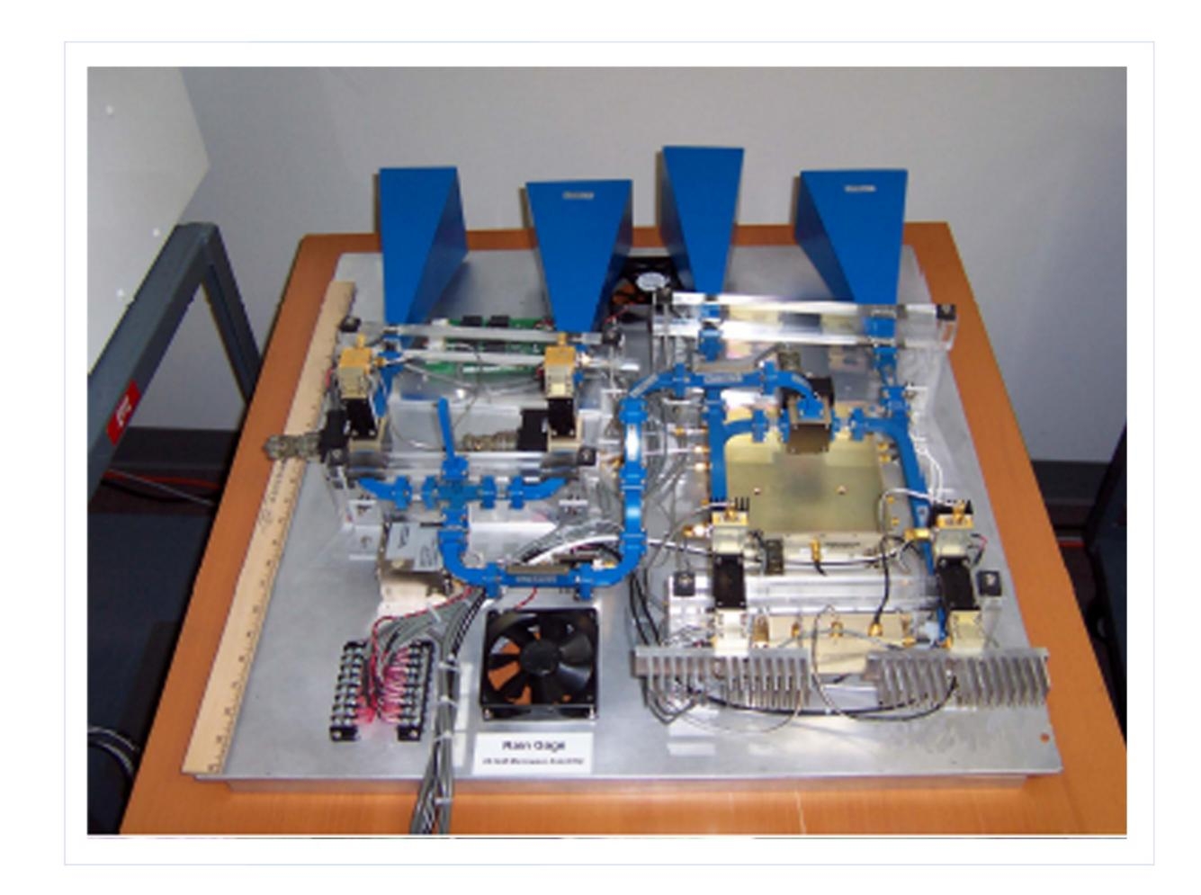
A novel, high-performance, and versatile instrument for monitoring various rain parameters has been developed. It consists of three flexible, multipolarization radar systems with extremely precise amplitude and phase calibration. The three radars operate at 13.6, 25, and 37 GHz and are completely software controlled.
